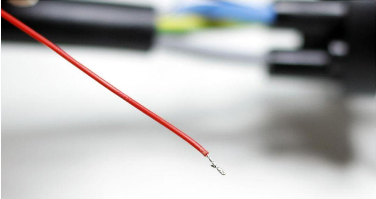
Slide a piece of shrinking sleeve over the small cable wires and crimp the small terminals on the wires:
